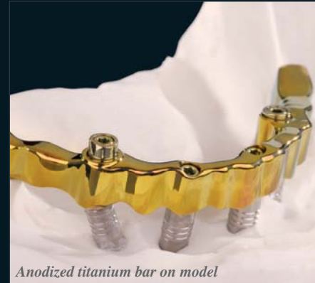
Titanium bar – CAD/CAM milled from Titan 5
