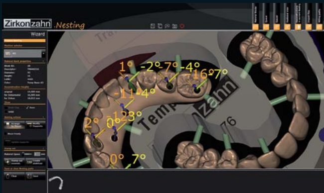
Nesting of the mandibular provisional and the temporary maxillary resin teeth in the Temp Basic block.
