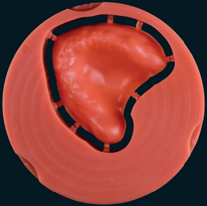
Palatal plate milled from Temp Basic Tissue
