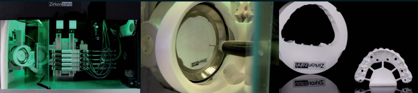
Milling the mandibular Prettau® Bridge using the M5 five-axis simultaneous-function milling unit.
