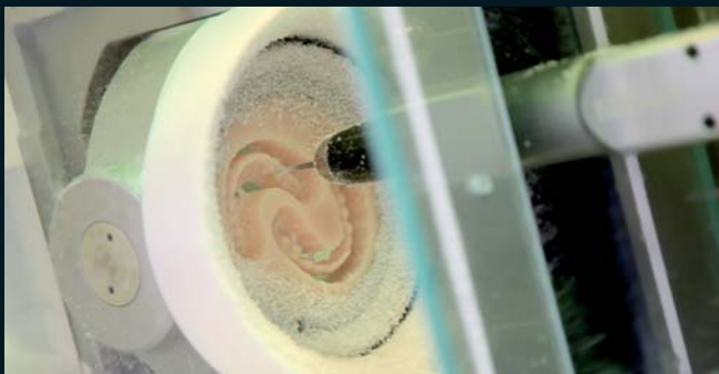
Milling the designs using the M5 five-axis simultaneous milling unit.
