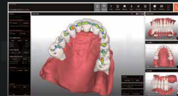
Fig. 7: Zirkonzahn.Modifier identifies the tooth contact relationships automatically. If something is changed in the upper or lower jaw, the effects on the antagonist are always carried out automatically by the software.
