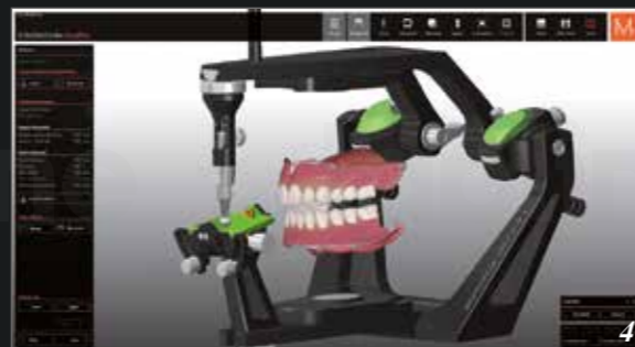
Fig. 4: The new articulator permits to perform all natural jaw movements and reproduce different occlusion concepts, such as that of sequential movements according to Slavicek.
