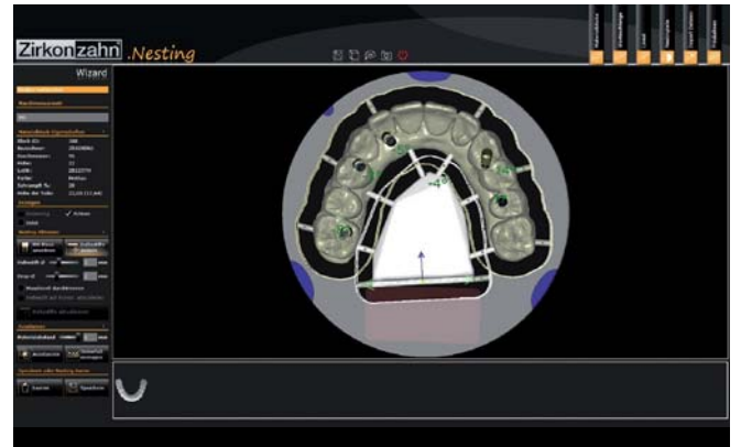
31 Positioning the finished virtual maxillary wax-up in the Prettau® Zirconia blank 22 mm in height. A sintering support for distortion-free sintering is also provided.
