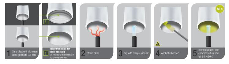
2. Preparation of the Zirkonzahn titanium bases
