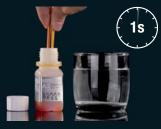
Immerse the Prettau<sup>®</sup> Anterior<sup>®</sup> crown with a pair of plastic tweezers for approx. 1 sec. into the liquid
