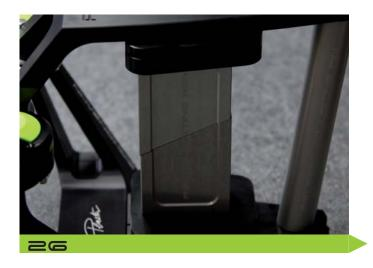
... the two halves of the Adjusting Key PS1 should lie smoothly on each other. Should that not be the case, it is an indication for a distortion of the upper base plate. If this occurs, the upper base plate should be removed and glued again with the Adjusting Key PS1.
