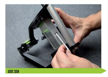
Loosen the two screws of the Adjusting Key PS1 ...
