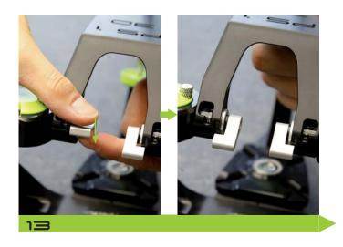
In case the angle is not at  $0^\circ$ , it can be corrected by rotating the axis and then turning the levers.
