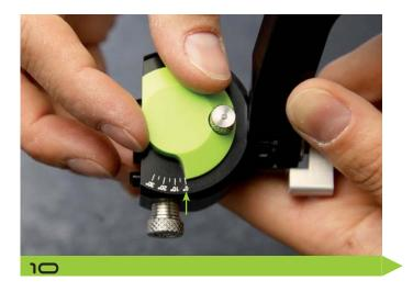
**ATTENTION:** before properly fixing the screws, make sure that the angle of the lateral condylar guidance is positioned at  $0^{\circ}$ !
