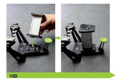
Mount the Adjusting Key PS1 on the Splitcast-plate of the articulator.
