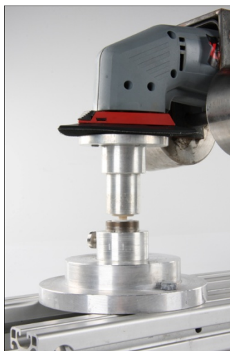
Figure 5 shows the contact arrangement between material sample and the indenter.
