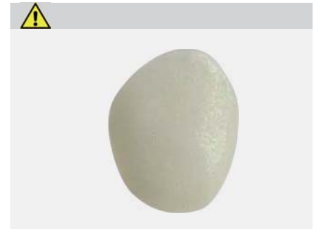
CAUTION Too low temperature!
