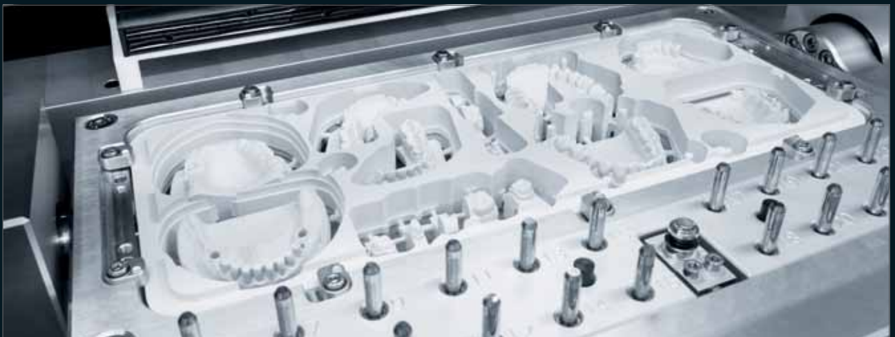
By using the extra large Model Blank M4 up to 20 full arches can be milled in a single milling process in the M4 Wet Heavy Metal milling unit.
