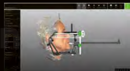
The digital acquisition of patient information using the PlaneSystem® and the Face Hunter 3D facial scanner permits the improvement of predictability, reproducibility and accuracy of the treatment, in order to manufacture patient-specific prostheses.
