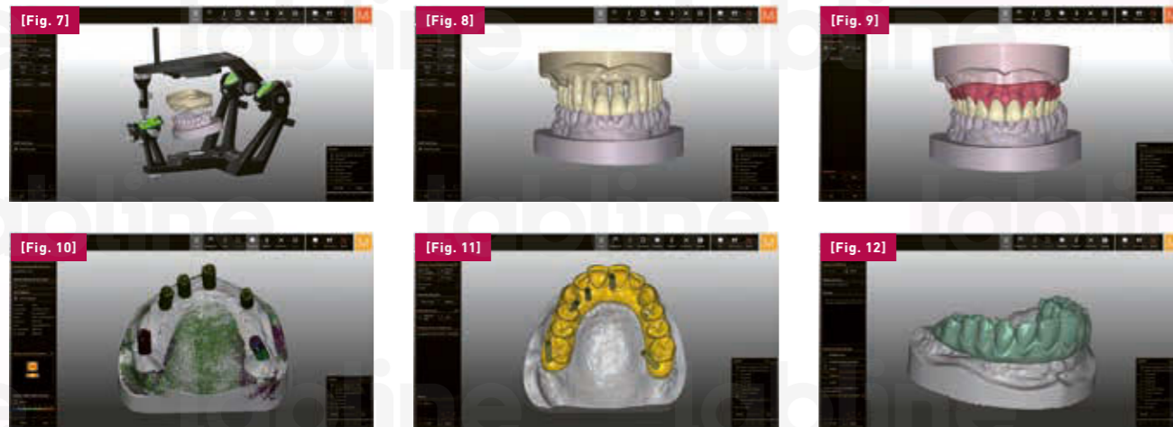
[Fig. 7] The models transferred to the add-on software and virtually articulated to reproduce the individual dynamic movements
