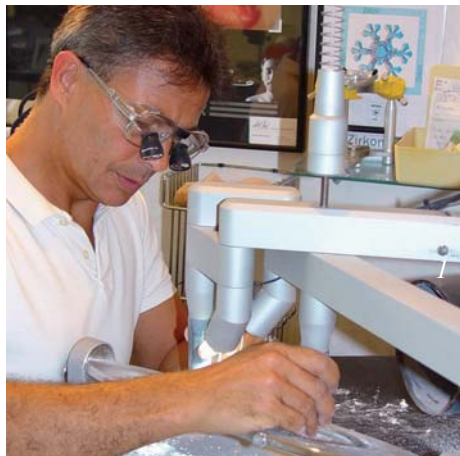
Copy milling procedure in 5 axes
